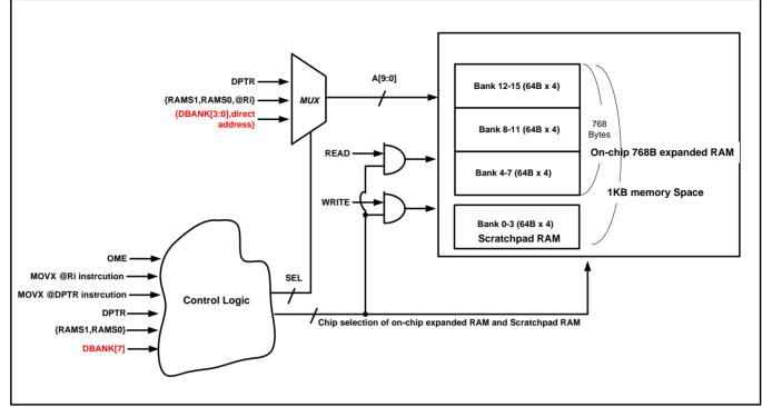
Fig.3-4: Access on-chip expanded RAM and scratchpad RAM with both in single 1KB addressing space scheme
