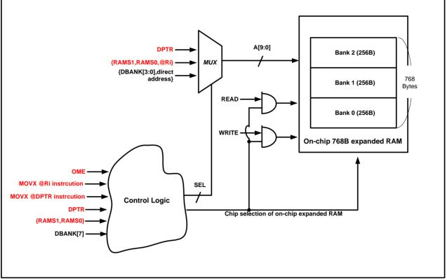
Fig. 3-3: Access on-chip expanded RAM scheme
