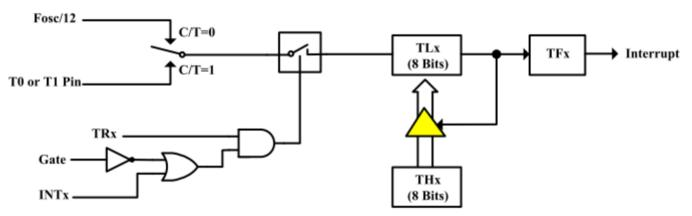
Fig. 6-3: Mode 2 8-bit auto-reload Counter/Timer operation.
